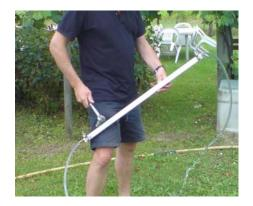
fig. 1: flush the hose and attach it to the Cu tube. Fix the hose on the Cu with a clip fig. 2: hit the aluminium rack with (most convenient here with the rachet)
